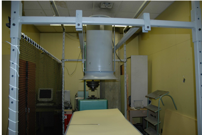
Figure 2.5: The “Open” vortex generator device showing the axial duct fan, the frame, and test table.
